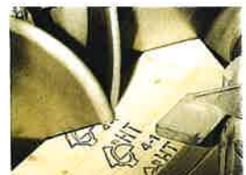
Accurate machine cut rafters make a tight joint for maximum strength and precise construction.
